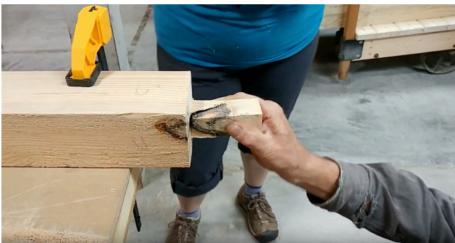
Figure 2. Helen finds a knot when carving this tenon for a wall stud. The knot's placement meant the tenon would not be strong enough, so this piece was reused for another purpose.
