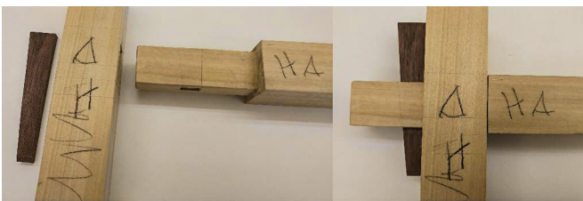
Figure 4: A tusk tenon taken apart (L) and together (R). The markings denote orientation so gravity can help keep the joint secure despite daily racking forces.
