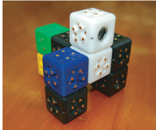
Figure 8. roBlocks construction kit for modular robotics
