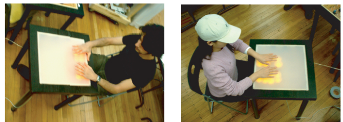
Figure 3. Each Telepresence Table translates shadow patterns into light and transmits them to the other table.
